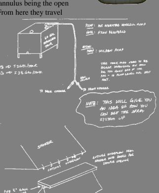
To help meet the regulatory requirements associated with discharging the cuttings to the sea (if applicable), 8 - 10, stainless steel nozzles are arranged to cover the spent materials traveling path, prior to over-board discharge. The nozzles are placed across each shaker screen, the ditch and once again in the actual disposal chute to the sea floor.
